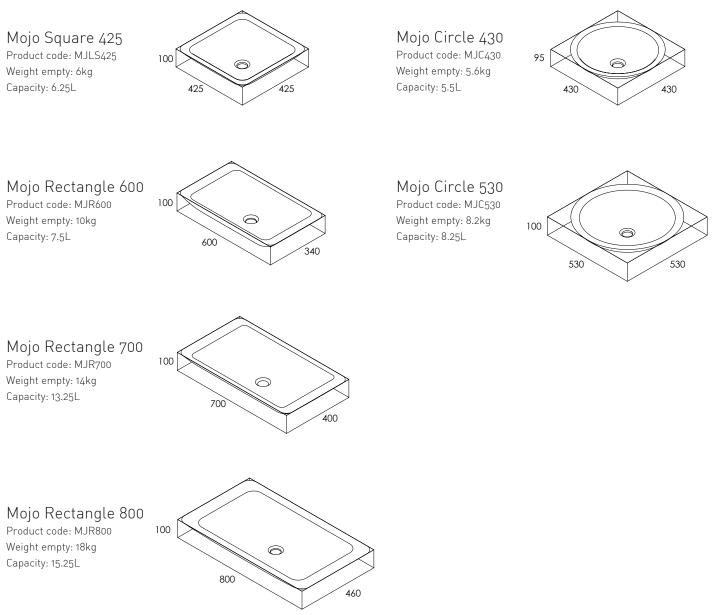
Tap holes: N/A Waste: 32mm no overflow Plug & Waste not included Measurements can vary +/- 5mm All bathware supplied in a semi gloss finish
